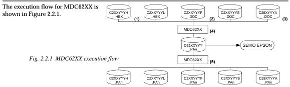
(1) Preparation of program data files (C2XXYYYH.HEX and C2XXYYYL.HEX) Prepare the program data files generated from the Cross Assembler (ASM62XX).
